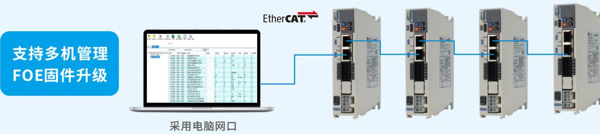
The diagram illustrates multi-machine management via Ethernet network. A laptop is connected to a series of four DM5 series bus type drives. The laptop screen displays a software interface for multi-machine management. The text '支持多机管理 FOE固件升级' (Support multi-machine management FOE firmware upgrade) is shown in a blue box. The text '采用电脑网口' (Using computer network port) is shown below the laptop. The text 'EtherCAT' is shown above the drives, indicating the communication protocol used.
