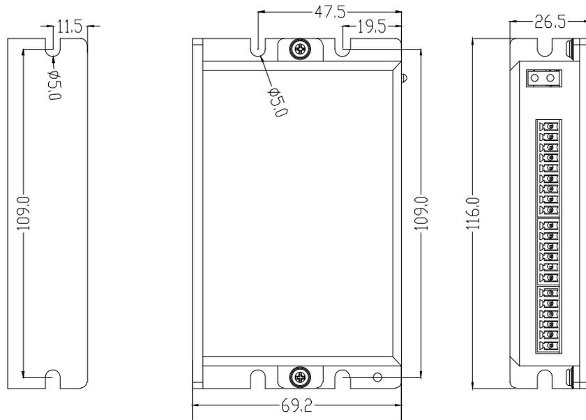
CL42C V2.0/CL57C V2.0安装尺寸图
